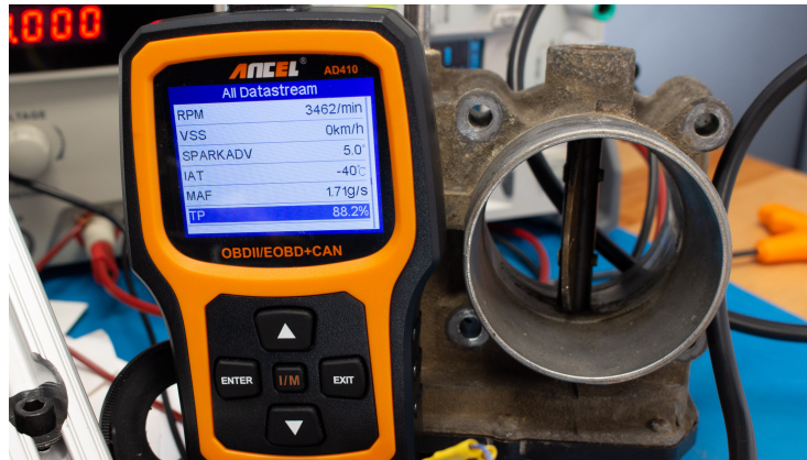
Figure 14: The ECU after an EMFI based fault caused some error where the throttle is commanded to become fully open.
