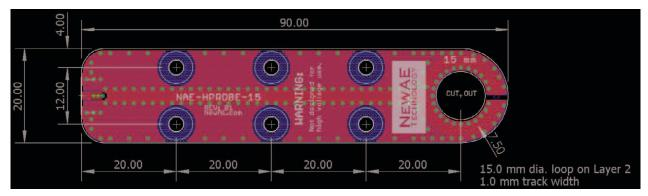
The above shows all four layers of the PCB used in the planar H-Field probe. The specific layers are shown on the following page.
