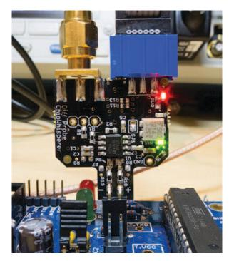
The supply voltages of the differential probe must be at least 2V above/below (for +V & -V respectively) the common mode voltage. The Probe Power Supply (CW503) provides a +/- 8V supply, allowing you to use the probe on any reasonable shunt inserted into VCC and GND.
