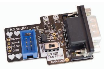
CANoodler is a simple CAN (not CAN-FD) interface, which provides logic-level 3.3V output. It's designed to be used with microcontrollers that have CAN blocks inside them, and in particular uses a pinout present on some ChipWhisperer CW308 (UFO) Target boards.
