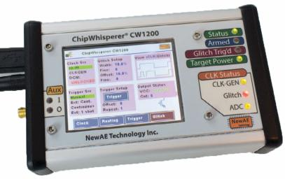
The ChipWhisperer-Pro has been designed to remain compatible with existing ChipWhisperer-Lite interfaces, but adds new features thanks to a larger internal FPGA.
