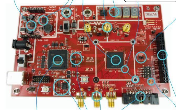
Custom USB interface provides API to directly read/write into FPGA memory space, along with FPGA configuration in 2 seconds.
