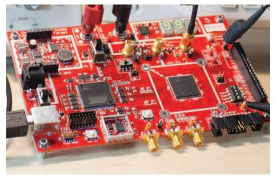
The CW305 is an advanced target for performing power analysis & fault injection attacks against hardware cryptographic functions implemented in FPGAs.
