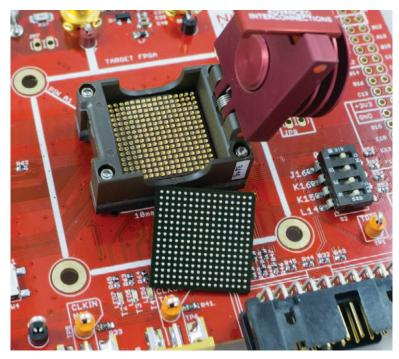
When closed, the socket has a heat sink on top of the FPGA. Note the socket prevents usage with an EM probe or similar.
