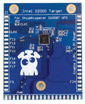
The CW308T-D2000 target series allows experiments on the unique D2000 target from Intel. This target has an X86 core in a microcontroller body. You can experiment with various aspects of the device and see how something besides an Arm device performs!
