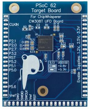
The PSoC62 board features the CY8C6247BZI-D44 from Cypress Semiconductors. This device features multiple secure boot features, and a seperate Cortex-M0 "security code" in addition to the Cortex-M4 "main processor.
