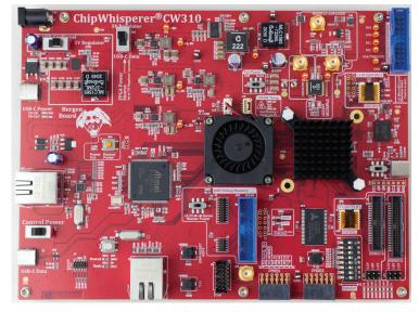
This CW310 Bergen Board is a Kintex K410T based FPGA target. The large FPGA can implement version of the OpenTitan project, along with large SoCs and other designs.
