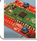
Solder the 2 push buttons. If you are mounting the Raspberry Pi Pico on pins, you may find it easier to solder the push buttons first.
